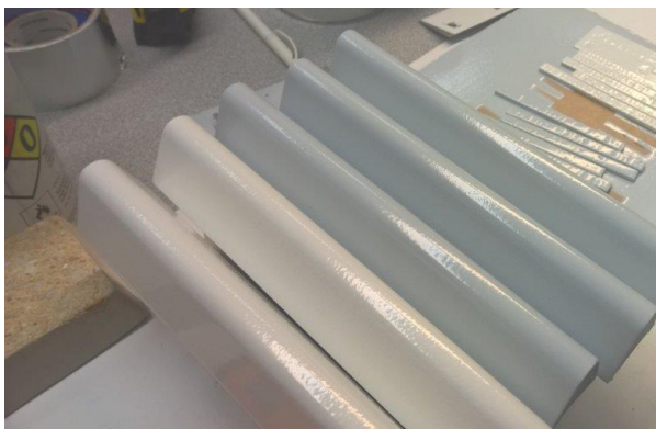
FIGURE 3: Scheme of rain erosion (RE) samples (A); Image of RE samples without coating and coated
