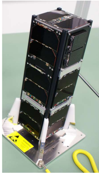
Figure 5, flight ready PEASSS satellite with visible in the left picture the 2 sun-sensors and in the right picture the 2 black pyro power generator elements
