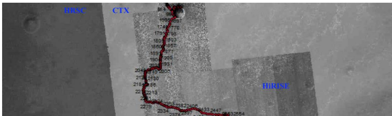
Figure 19: Final product: HRSC, CTX, HiRISE registration including corrected rover traverse
