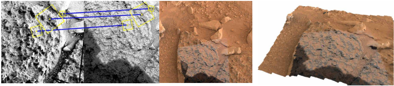
Figure 17: (left) Automated fusion of Mastcam and MAHLI 25 cm data, (middle) result 2D view and (right) 3D view
