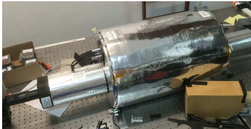
Instrument CHROMIS at the SST. The pipeline is the software that takes care of the data from the instrument.
