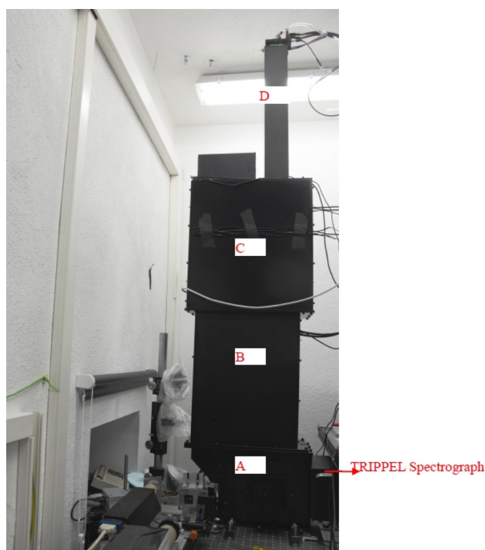
Assembled MiHI unit in front of the TRIPPEL spectrograph. A, B, C, D are the different sub-assemblies.
