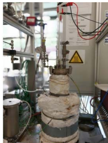
Figure 9. Electrochemical system developed by DLR within activities of WP15 to detect and analyse impurities in molten salts.
