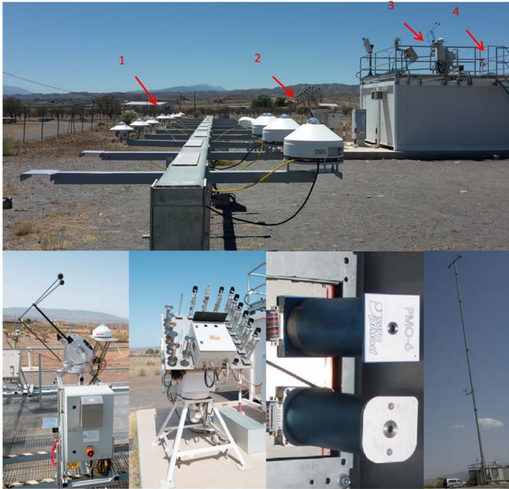
Figure 2. Top: Overview of METAS calibration setup (1: Pyranometer test bench; 2: Pyrhelimeters test bench; 3: Black Photon tracker with DHI reference; 4: cloud camera); Bottom left: detail view of Black Photon tracker; Bottom left centre: detail view of pyrhelimeter test bench; Bottom right centre: two absolute cavity reference pyrhelimeters located in the pyrhelimeter test bench's front cabinet; Bottom right: METAS wind mast (WP11).
