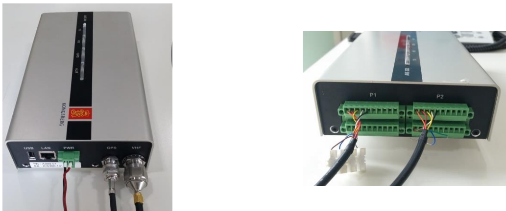
Figure 4: AIS 300 mobile station included in the TRITON prototype
