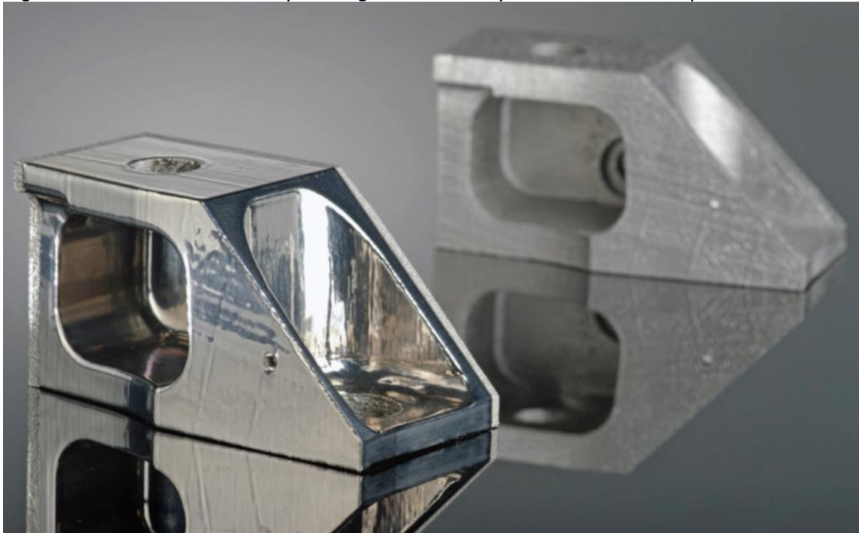
Figure 9 Fraunhofer ILT laser polishing of IN718 compared to Am as built part.
