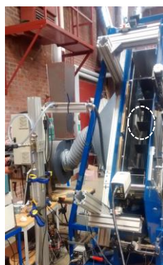
Cooled vane experimental set-up in the Chalmers linear OGV rig
