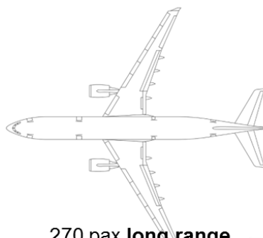
270 pax long range turbofan aircraft 6500 NM design range, 0.82 MN
