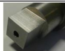
Cathode 2: Sphere contour (R6,5mm); frontal and lateral machining
