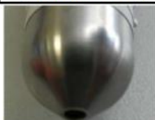
Cathode 2: Sphere contour (R6,5mm); frontal and lateral machining
