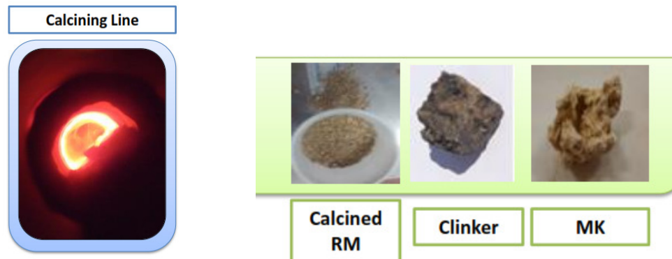
Figure 10. Example of calcines clinker raw meal, clinker and metakaolin obtained with Demonstrator's Setup
