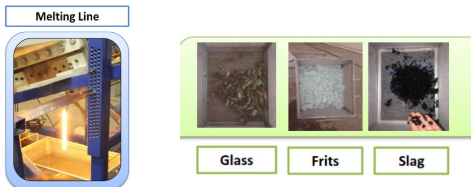
Figure 9. Example of glass, frits and slag cement obtained with Demonstrator's Setup.
