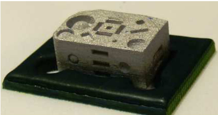
Test geometry demo component fixed in its placeholder in the Hyproline
