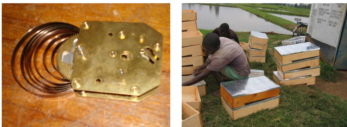
Figure 13: Clockwork feeder components and assembly
