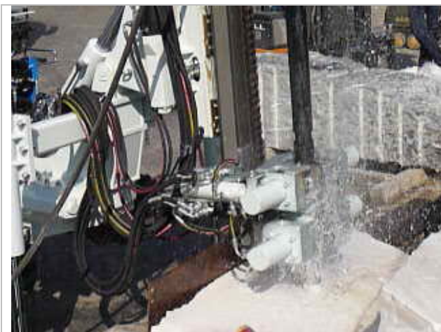
Figure 3-25: Drilling test on marble and granite
