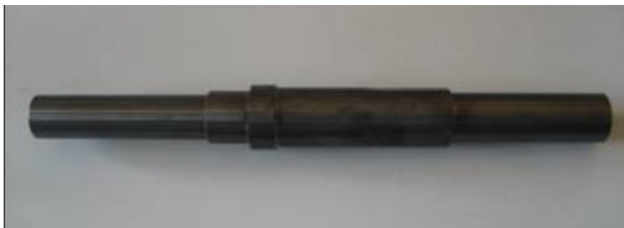
Figure 1-2: Piston with chromising - DLC
