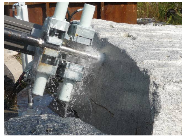
Figure 3-25: Drilling test on marble and granite
