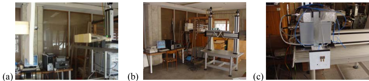
Figure 3-8: SAR imaging System with mechanical scanner
