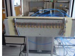
Figure 3-10: MIMO-SAR system: array installed on scanner
