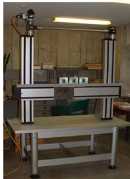
Figure 3-1: Mechanical scanner with three movable antennas
