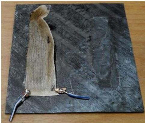
Figure 23 Disassembled omega stringer from skin
