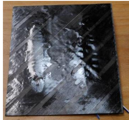
Figure 23 Disassembled omega stringer from skin
