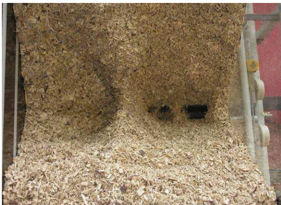
Figure 7: Point of first bridge collapse (“OW1”) with a wood chip fuel sample
