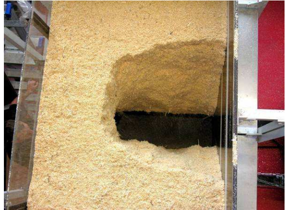
Figure 8: Point of 50 %-bridge collapse (“OW50”) with a saw dust fuel sample
