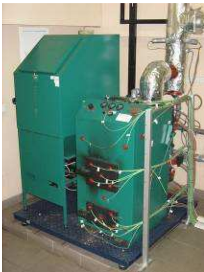
Figure 6: A Latvian pellet boiler used in the tests as installed in the tests rig.
