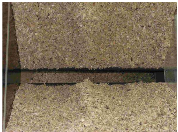
Figure 9: Point of 100 %-bridge collapse (“OW100”) with a wood chip fuel sample
