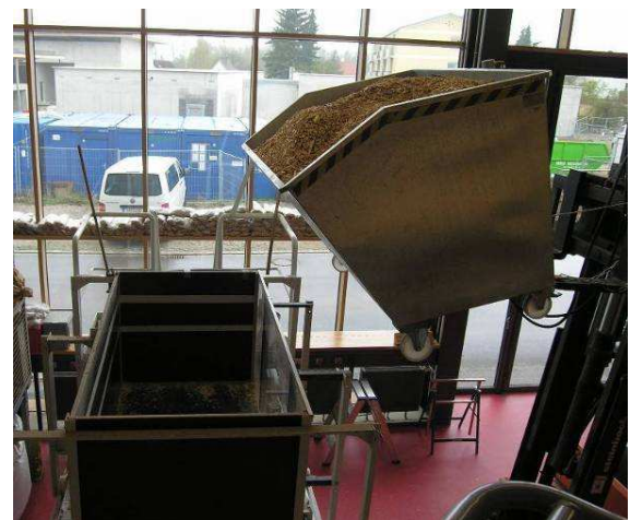
Figure 6: Filled tilting container mounted on a fork lifter before dropping the sample into the tester The sample volume was fixed to 1.65 \text{ m}^3 for all tests. The sample was homogenized before the tests; this
