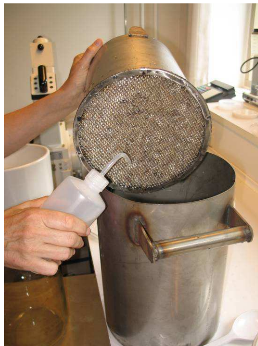
Figure 1: Gently tip the inner container and rinse any particles of the bottom of the inner container into the outer container.
