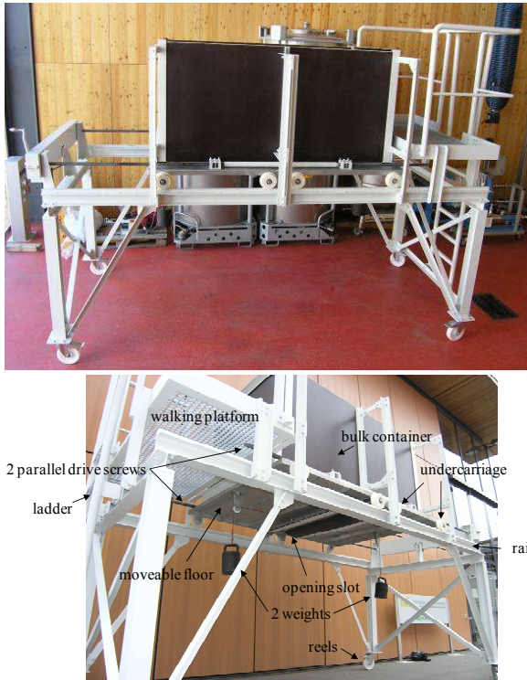
Figure 4: The TFZ bridging tester
