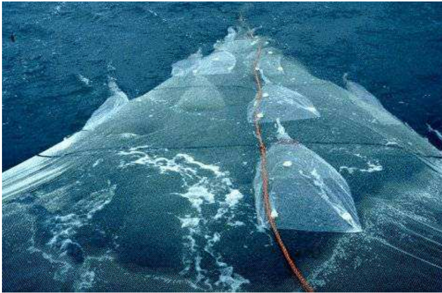
Figure 9. Particular of the net bags mounted on the different parts of the trawl body in the sea trials carried out to evaluate current gear selectivity of single- and pair-trawlers.
