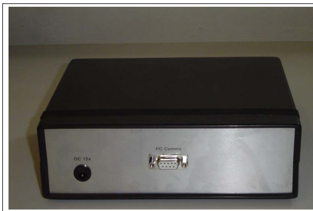
Figure 141. Rear of ELISHA electronics with serial communications port for connection to PC and power supply connections.
