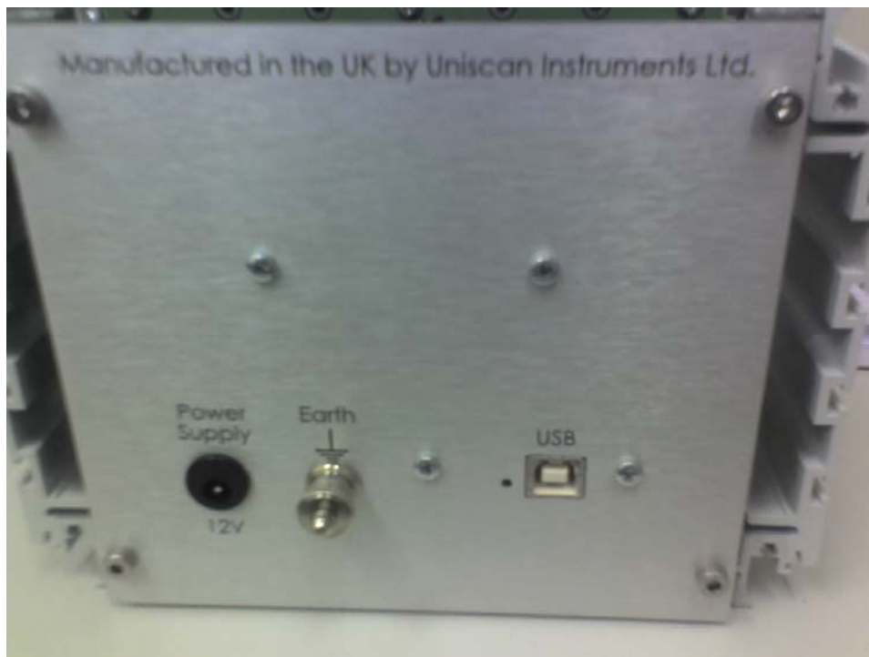
Figure 223. Rear of ELISHA electronics with USB communications port for connection to PC, power supply jack and earth stub.
