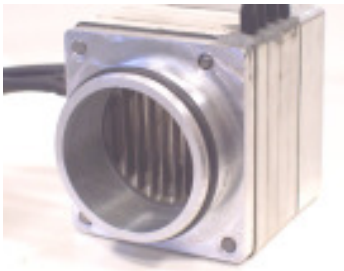
Figure A1.2 Prototype of the electrical air heater used at the inlet of the intake manifold of the engine.
