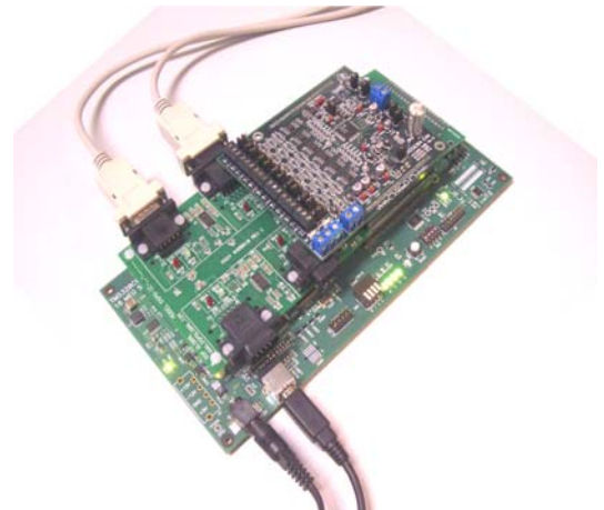
Figure 4.1.2. The Digital Signal Acquisition and Processing Hardware (DSP TI 6713 EVM board)
