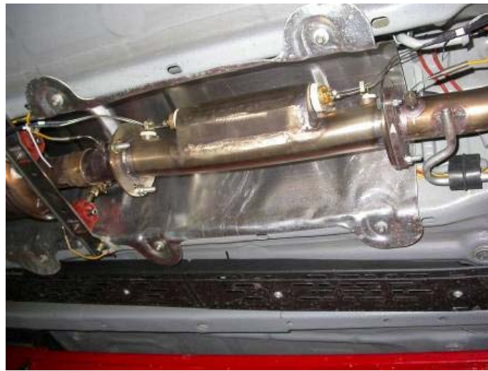
Figure 5.2.1 Photograph of The UV Optical Fibre Gas Sensors Mounted Underneath the Vehicle.
