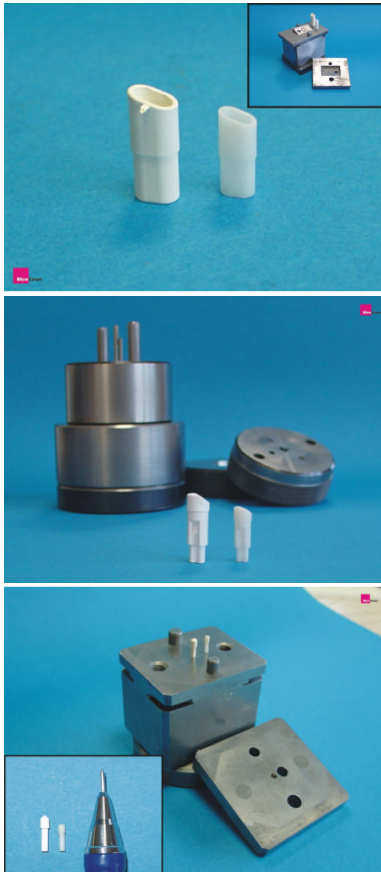
Fig. 2.4-22: Prototypes from nano zirconia for medicine technique – left part as fired, right part as sintered
