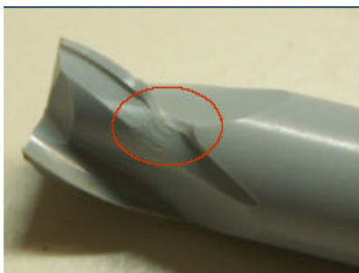
Fig. 2.8-7: Test of tool No 13 from nano ceramic 022406-2
