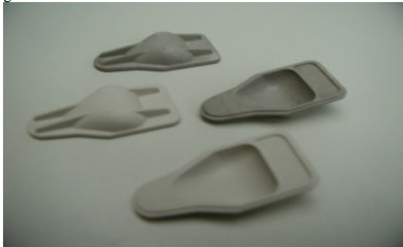
Fig. 2.3-1: Valve from nano Si 3 N 4 material produced by PIM (high pressure injection moulding)
