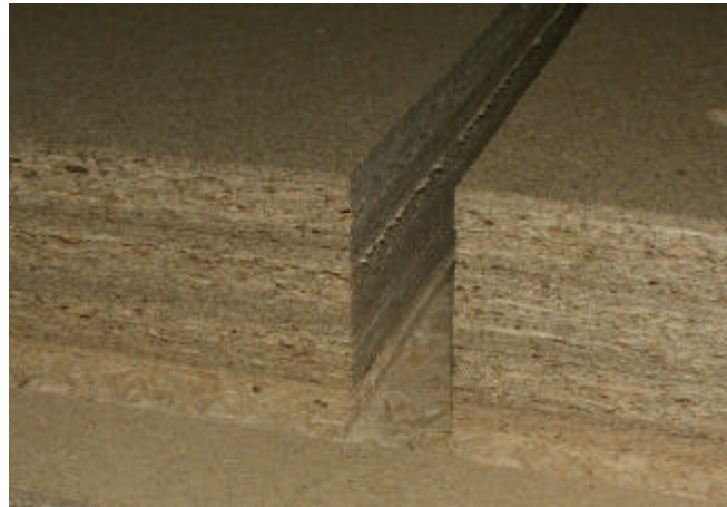
Fig. 2.8-1: Chipboard (3 layer x 16mm) and the used test conditions: Router diameter Ø20mm Spindle speed: 16.000 rpm machine: CNC 3 spindle machine from SCM Feed rate per teeth: 0,1875mm/U vf.: 3m/min (very slow, because of 3 layers) cutting distance: 368m (Diamond 5000m)
