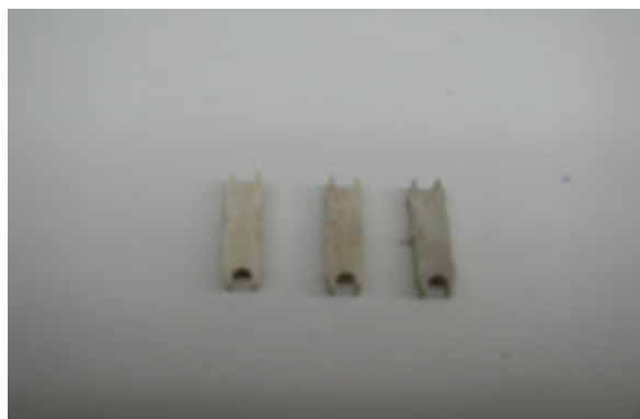
Fig. 2.4-3. simple part from zirconia plasma powder shaped by PIM
