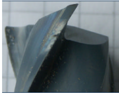
Fig. 2.8-8: Test of tool No 4 from nano ceramic 010906-1
