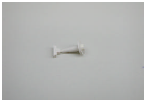
Fig. 2.4-4: Second part from zirconia plasma powder shaped by PIM
