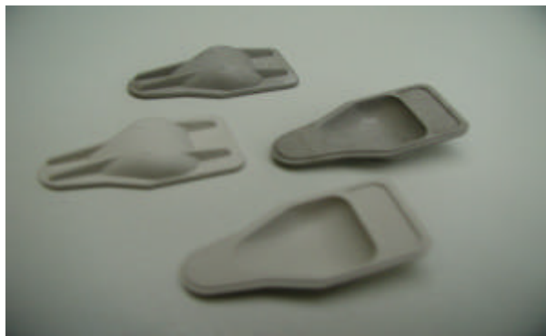
Fig.2.5-13: Sintered prototypes (valves) using a mixture containing 50 % nano \text{Si}_3\text{N}_4 powder
