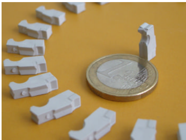
Fig: 2.6-8: Saw teeth from nano \text{Si}_3\text{N}_4 shaped by MPIM
