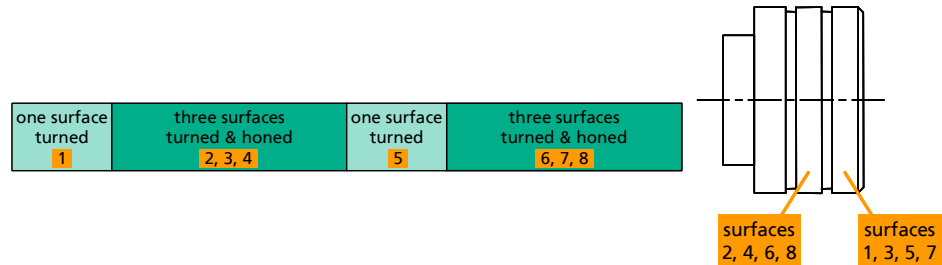
Fig. 19: Proceeding of the TAF tests for one batch
