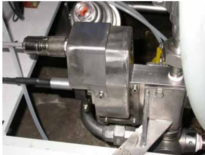
Figure 4 – Details of the EDY system: VOPS probes /1
