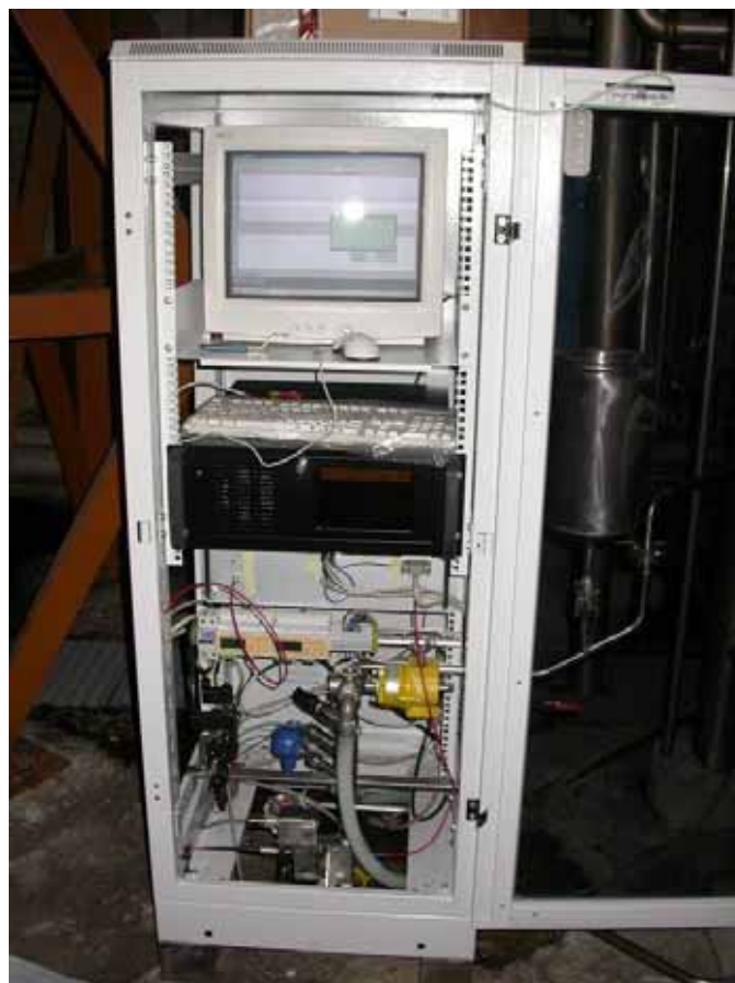
Figure 8 – Details of the EDY system: rack with control PC and probes: prototype installed in Italy
