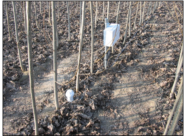
Figure 9 and 10: Spanish prototype inside the container and sensor probe with the battery surrounded by poplars.
