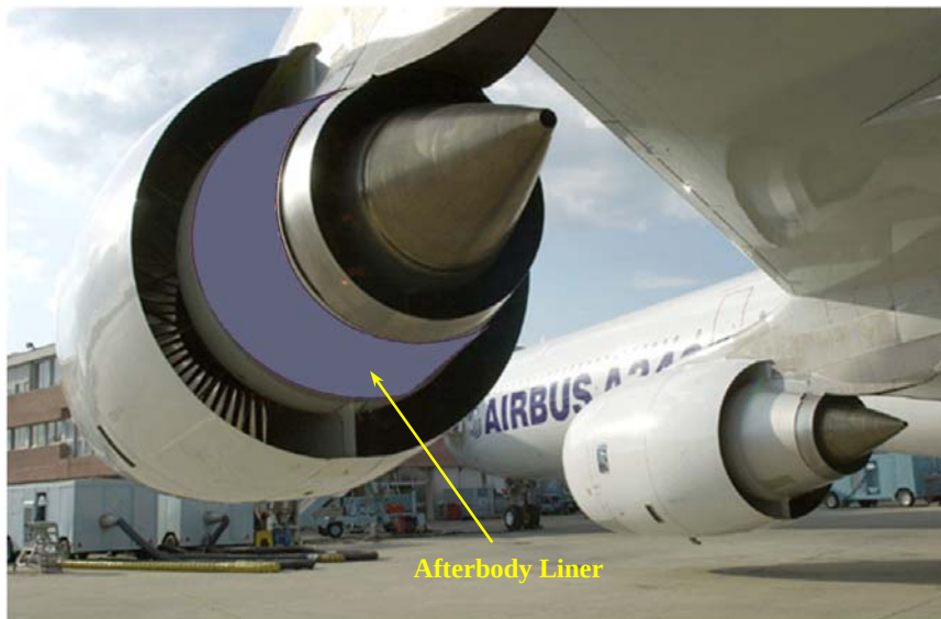
Figure 1.9: Possible application of Afterbody Liner acoustical treatment on a typical turbofan engine
