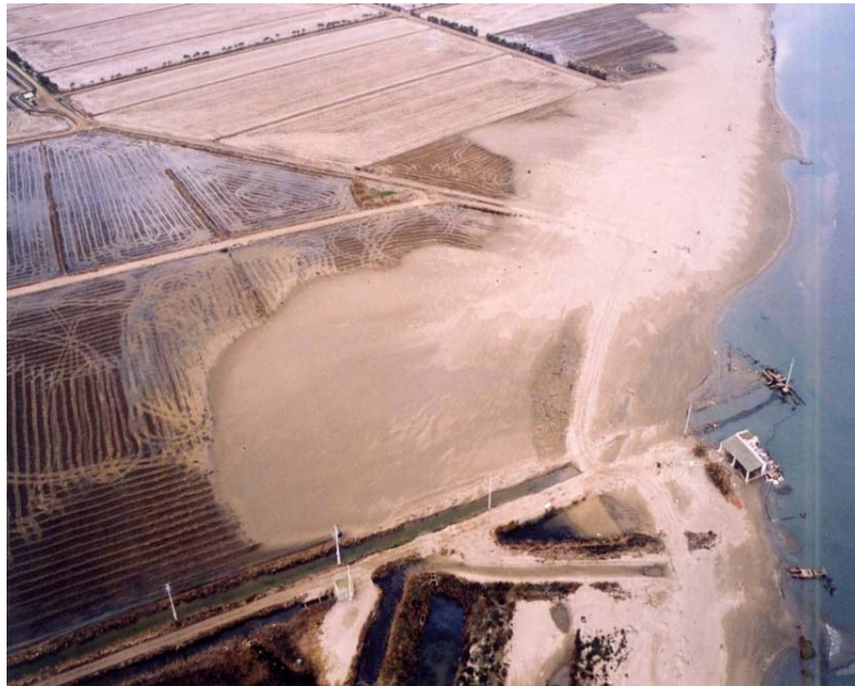
Figure 43. Illustration of marine flooding and associated vertical accretion in the Ebro delta (from UPC work).
