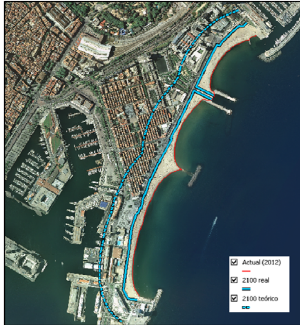
Figure 41. Present and projected (year 2100, assuming an average sea level scenario from RCP4.5) public domain baseline for the Barcelona littoral. The present limit has been associated to the promenade boundary while the future limit corresponds to the shoreline projected to the year 2100 assuming flooding and no shoreward migration. The geometric projection considering a given sea level rise leads to a line that should be considered as reference since the actual boundary will be conditioned by human responses (adaptation) which may counter this sea level induced changes partially or totally.
