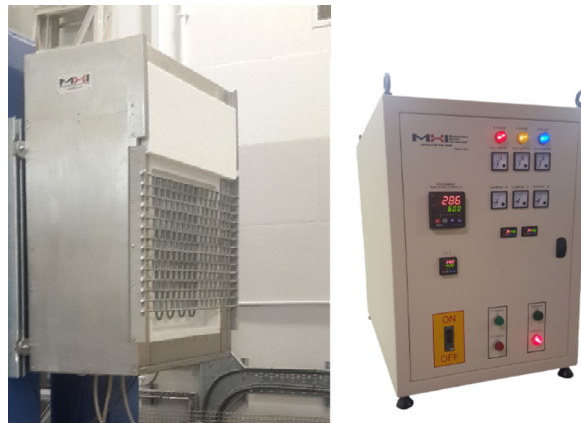
Figure 26 Vertical radiator and control unit
