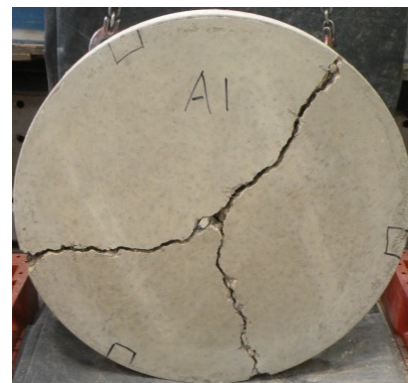
Figure 15 SFRC slab after flexural testing
