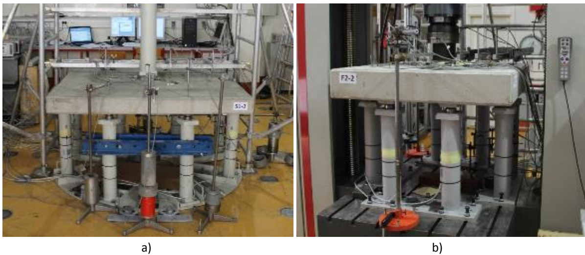
Figure 18 Test setup for: a) slabs; b) footings
