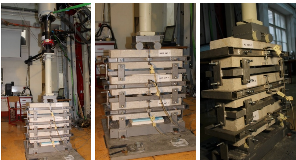
Figure 19 Fatigue test setup
