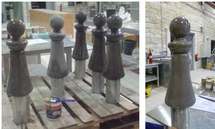
Figure 32 Safety road poles cast with steel fibre-reinforced rubberised concrete
