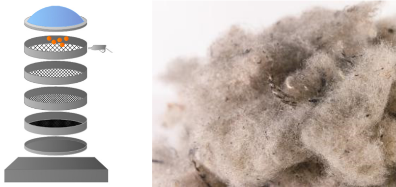
Figure 2 a) Schematic representation of RTPF cleaning device, b) sorted RTPF after cleaning
