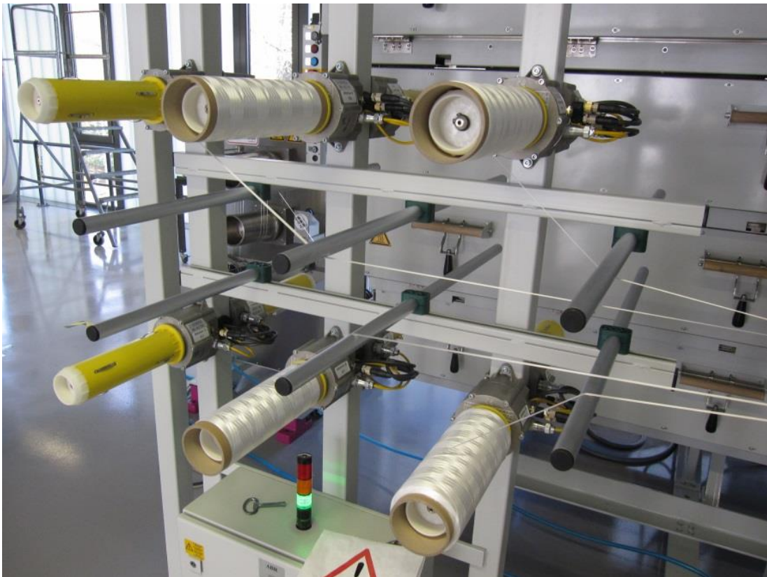
Figure 2 Joining of PE-precursor fibers in two steps from 0.3K up to 12K precursor fiber
