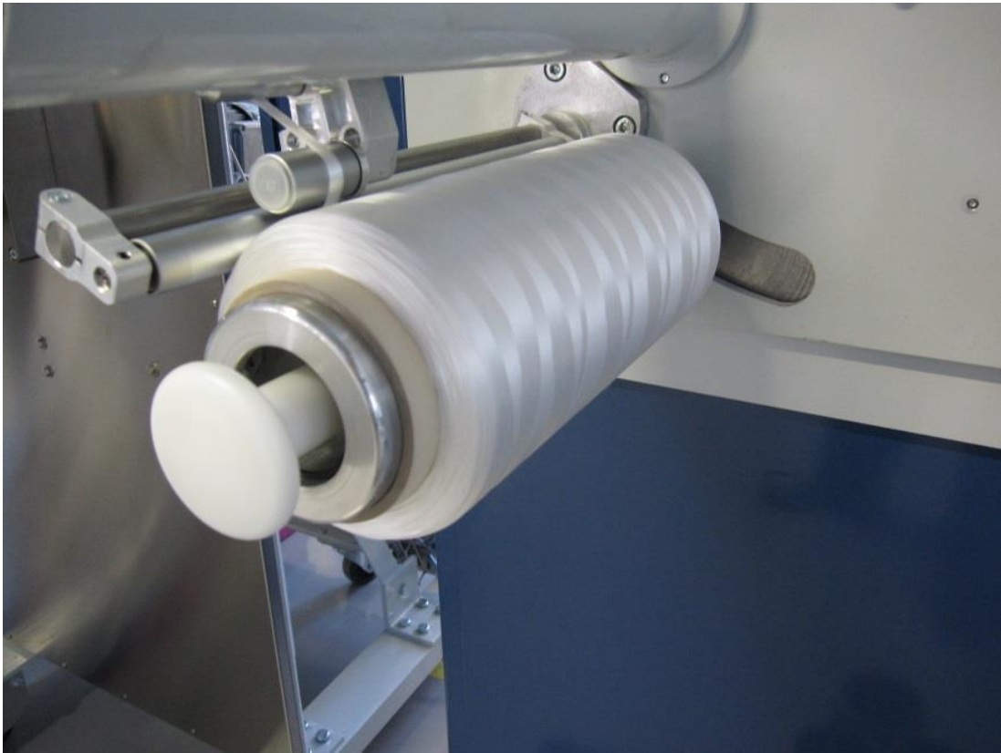
Figure 3 Winding of 12K precursor fiber
