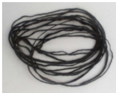
Figure 5: Samples of carbon fibers with lignin (tow and yarn)
