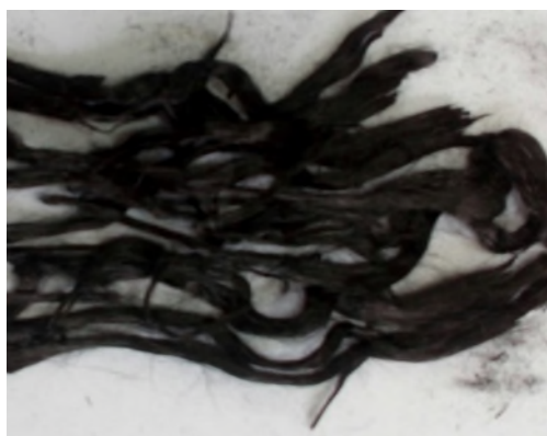
Figure 5: Samples of carbon fibers with lignin (tow and yarn)
