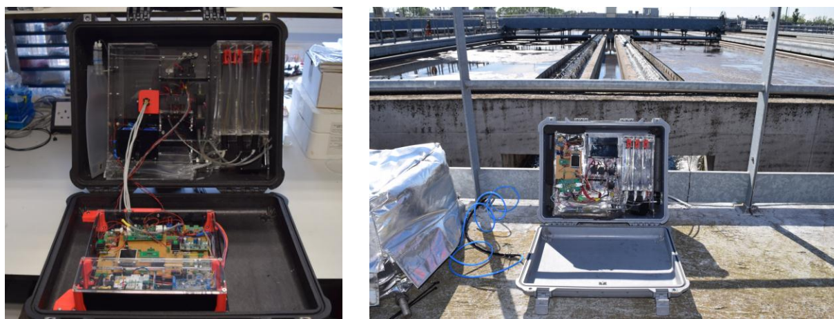
Figure 7 Fully-functioning autonomous nutrient analyser developed by DCU (left) and in deployment (right) at a waste water treatment plant in Milan (organized by UMIL and DCU)
