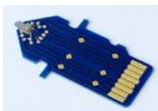
100kHz piezo-cantilever for gas detection
