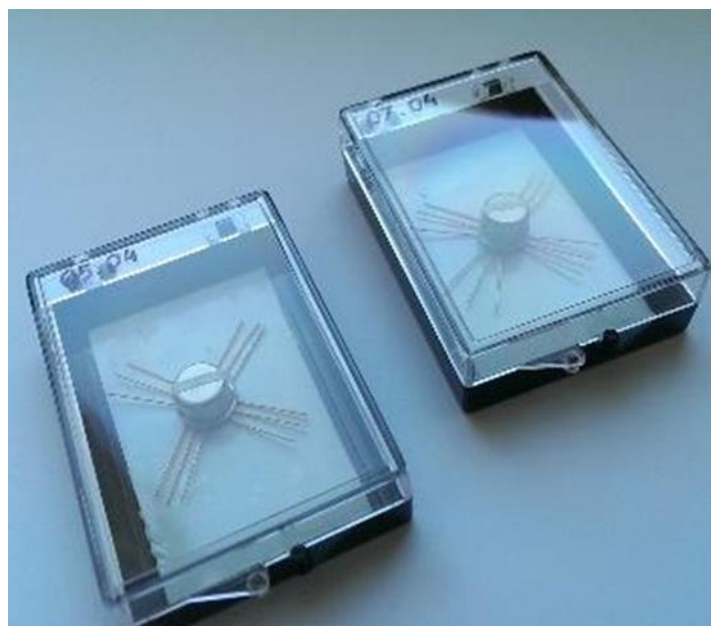
Figure 16 Spectrometer sensors, bonded in TO12 packages.
