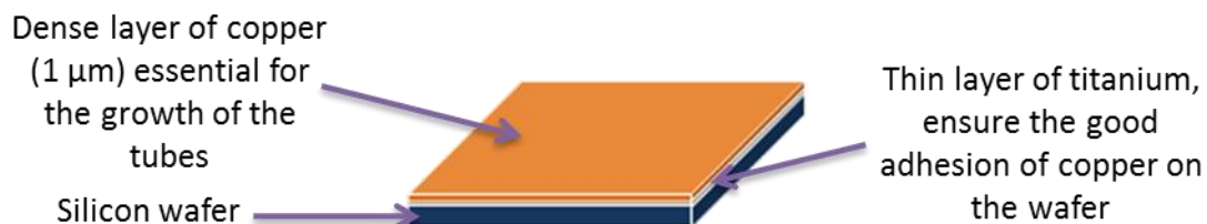
Figure 98 Preparation of silicon wafer for synthesis of CuO nanotubes.
