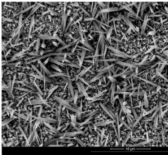
Figure 105 SEM image of CuO nanotubes synthesized on a cantilever membrane before final etching procedure.
