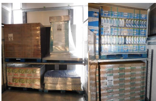
Figure 2-22: TRANSFORMERS Load Optimisation Trailer: Flex Floor Optimally Used
