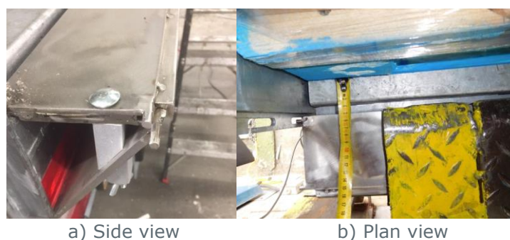
Figure 2-14: Load Optimisation Trailer: Collapsible Docking Plate Support
