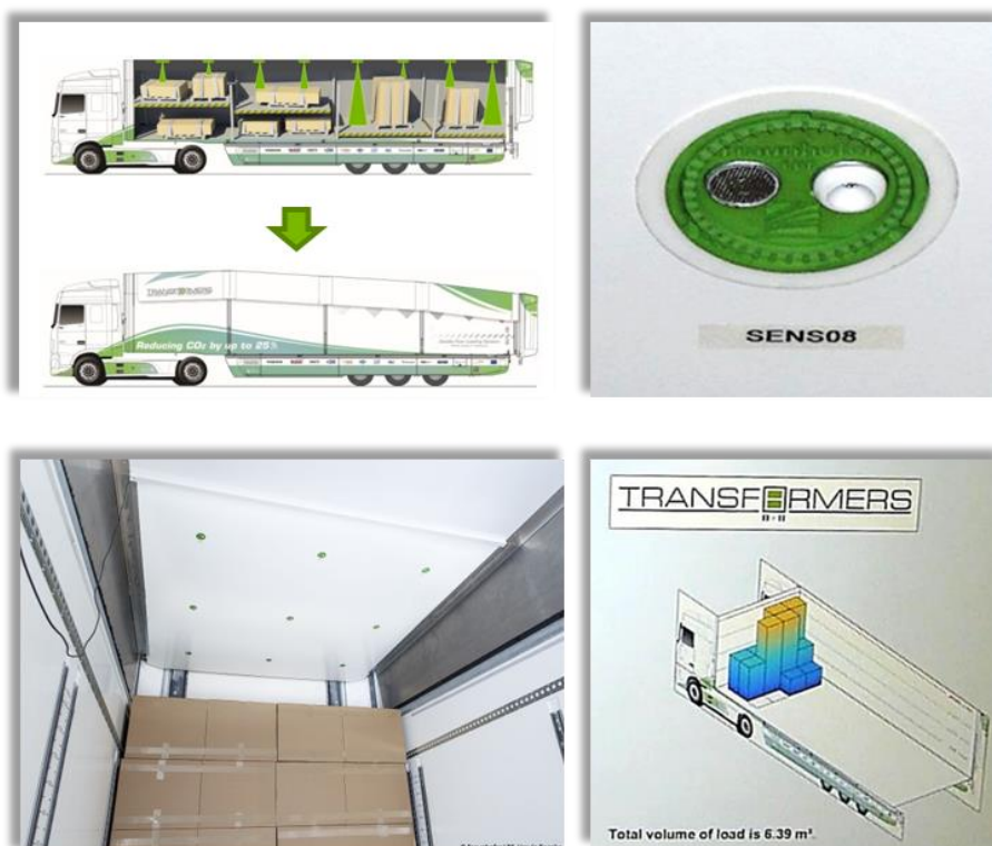
Figure 2-17: Load Optimisation Trailer: Load Volume Indicator System
