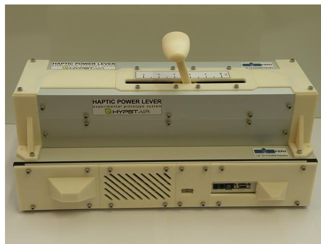
Figure 10: HYPSTAIR experimental prototype of the haptic power lever by University of Maribor
