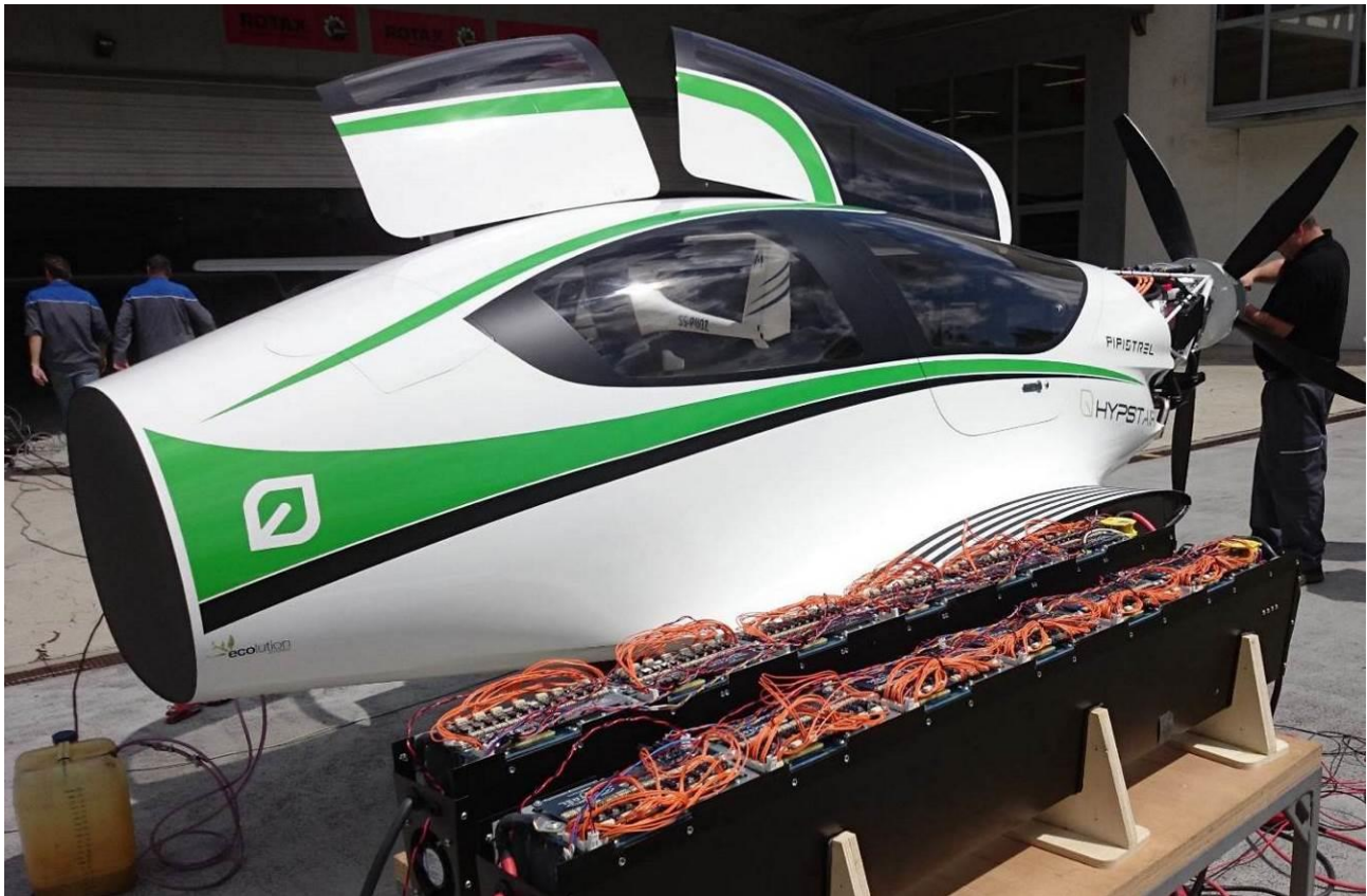
Figure 17 The HYPSTAIR propulsion battery developed by Pipistrel
