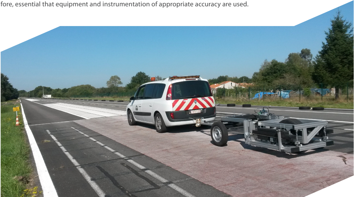
Figure 5. Trailer-based rolling resistance measurement method; an example of the force-based trailer (BRRC) performing measurements during the round robin test in Nantes
