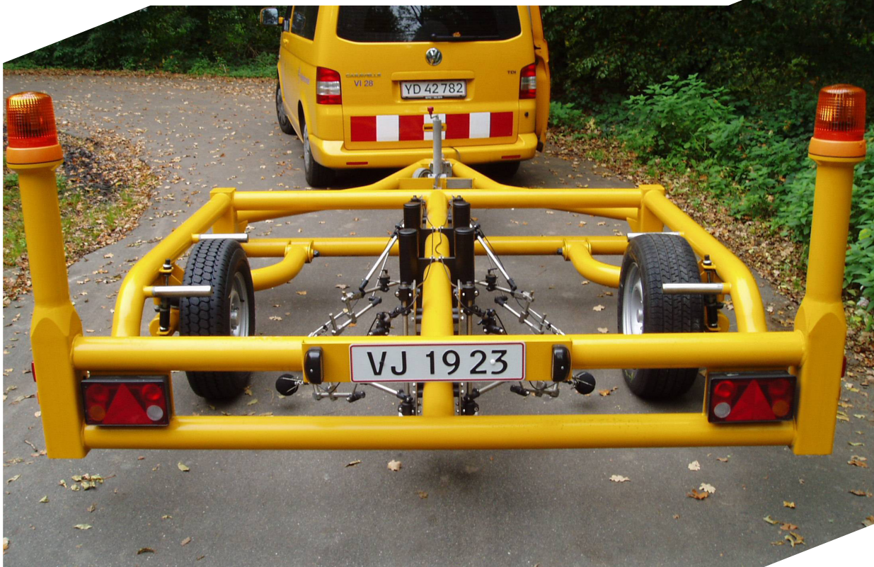
Figure 3. Equipment for CPX measurements: top – an example of an enclosed trailer (AIT); bottom – an example of an open trailer (DRD)
