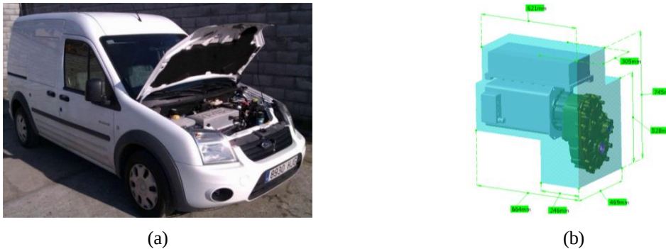
Figure 20. (a) Azure Transit Connect van; (b) Available space for the integration of new elements (original motor & inverter shown in blue).
