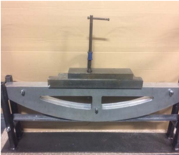
Figure 36. Positioning of stage 1 (semi-cured) profile under the forming tool (supported by the frame, left) for stage 2 processing. The frame is placed in an oven (right) to introduce the bending to the profile
