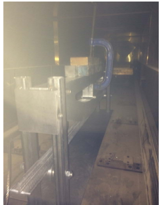
Figure 36. Positioning of stage 1 (semi-cured) profile under the forming tool (supported by the frame, left) for stage 2 processing. The frame is placed in an oven (right) to introduce the bending to the profile
