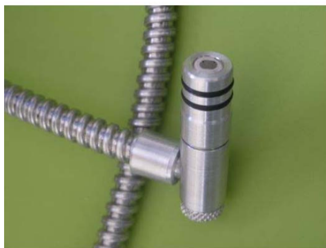
Figure 15. Dielectric sensors with embedded thermocouple for viscosity measurements.
