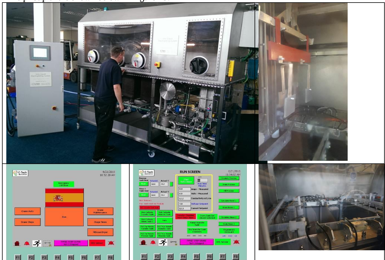
Figure 15: The SCAIL-UP Pilot Plant. From Top left clockwise: Main rig section incorporating the process tanks in an enclosure plus the electrical control panel, samples being lowered automatically into the plating tank, another view of the plating tank, main HMI operating screen, initial HMI screen.
