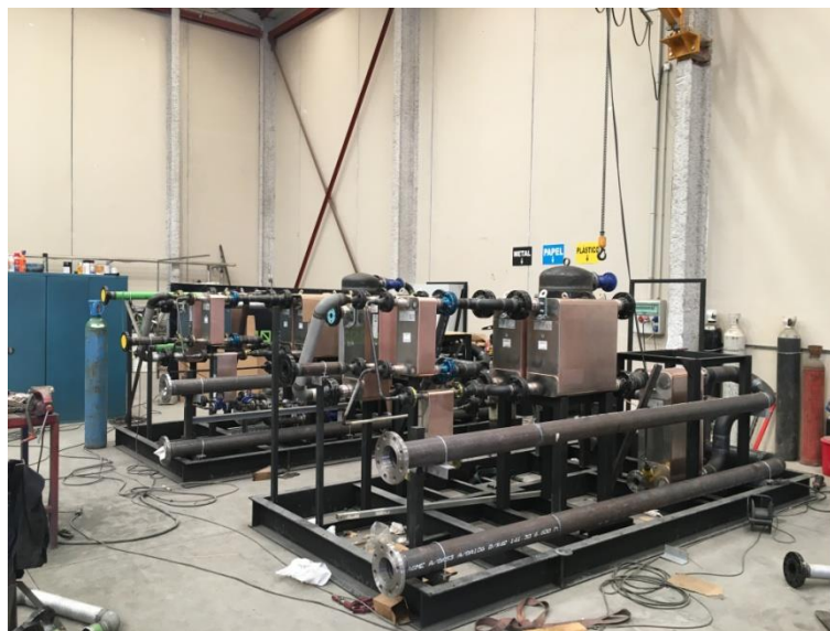
Turkey and Spain ORC units assembly process.
