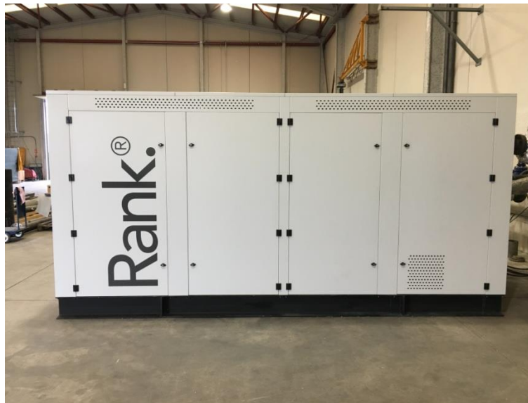
Figure 3.7: Liege ORC unit ready to be shipped.
