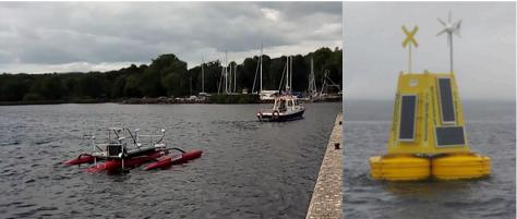
Figure 22 – The marine deployment vehicles for the BRAAVOO biosensor instruments, designed and fabricated by IDS Monitoring. Left and right, the data buoy. Middle, the USV in its "slave" configuration following a control boat.
