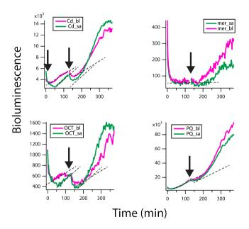
Figure 24 – Real sample analysis (encoded as "\_sa") in remote mode using the five-strain bacterial biosensor biochip with duplicate mode, in comparison to clean ONR7a medium (encoded as "\_bl"), plus injection of the calibration standard (at time 120 min.) Cd: cadmium biosensor. OCT: short-chain alkanes. PQ: oxidative stress. mer,  $Hg^{2+}$  sensor.
