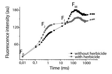
Figure 10 – Typical fluorescence kinetics of the photosystem II, as recorded on a Multilight Sensor (Biosensor srl.): 10 min dark, 11 sec of light at 127 arbitrary units, 10 sec recording. Samples or analytes were added directly to the free algal culture or to immobilized algae with prior exposition to light at 50  $\mu$ mol/m²s for 5 min. See main text for explanation of the major parameters  $F_{O}$ ,  $F_{V}$ ,  $F_{W}$ ,  $F_{M}$  and derivative calculations.
