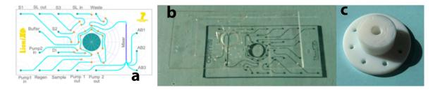
Figure 18 – Example of a rotary valve designed for the BRAAVOO biosensor microfluidics. a) Layout of the different possible fluidic connections. b) Glass chip with the etched channels. c) Teflon rotor with the connecting channels etched in its top, which fits the central hole in the glass chip.
