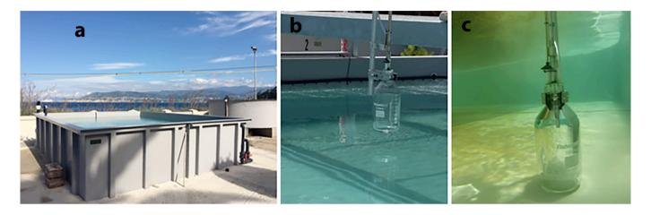
Figure 23 – Mesocosm facilities at Messina (a) used for the artificial oil spill sampling (b and c) to test biosensor's responses.
