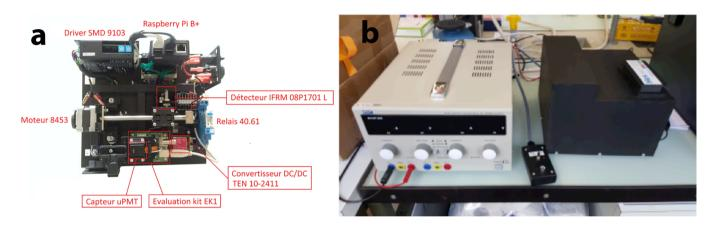
Figure 15 – The manual bacterial biochip bioluminescence reader produced for the BRAAVOO project. a) Inside stepper motor moving the 10 well biochip over the Hamamatsu microPMT detector. Raspberry PI controller for the motor, detector and data storage/transmission. b) Packed instrument on the right with power supply on the left.
