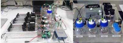
Figure 19 – Rotary valve control in the algal and nano-immuno sensors. Left, the stepper motor which controls the different positions of the rotary valve. Middle, integrated system with the syringe pumps, the reagents bottles, the fluidic connections and the Arduino control unit. Here shown for the nano-immunosensor unit. Right, Integrated fluidics for the algal sensor unit.
