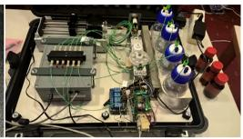
Figure 21 – The final connectable sensor instruments to the buoy and vessel. Left and middle, the nano-immuno aMZI platform with integrated fluidics and OSROM detector. Right, the algal sensor platform with integrated fluidics.
