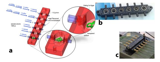
Figure 14 – The flow cell holder for the immobilized algae. a) Six parallel flow cells with internal filter structures enable the immobilized algae in calcium-alginate beads to remain inside while being exposed to a sample or regeneration solution. b) The RPDM-printed version of the six cages with the filter insets. c) The mounted closed flow cells with the fluidic connectors.
