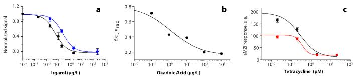
Figure 3 — Calibration curves for the nanoimmunosensor detection of (a) Irgarol, (b) Okadoic Acid, and (c) Tetracycline. a) black measurements: BiMW surface, blue: aMZI. b) BiMW surface; solutions prepared in PBS; anti-OA Ab at 0.5  $\mu$ g/mL. c) BiMW surface, tetracycline Ab at 1:6000 diluted (red) or at 1:3000 diluted (black line).
