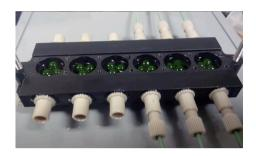
Figure 12 — Embedded and immobilized algae (green beads) in the photosystem II fluorescence sensor. The designed system has six parallel flow cells.
