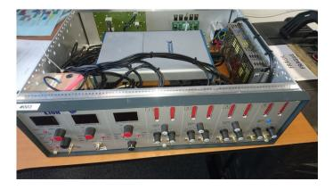
Figure 16 – The OSROM light source and detector unit for the aMZI and BiMW nano-immuno sensors.
