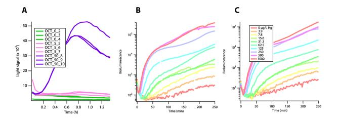
Figure 6 – Examples of freeze-dried biochip bioreporter performance. A) Replica testing of the 5150 reporter without (OCT\_0–2/3/4) or with octane (5  $\mu$ M, cyan lines; 50  $\mu$ M magenta). Triplicates in neighboring wells. B and C) Mercury bioreporters on a single chip either directly after freeze-drying (B) or after 1 month at 4°C (C). Concentrations as indicated.
