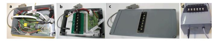
Figure 13 – Integrated fluorimeter instrument developed by Biosensor.srl to allow algal photosystem II fluorescence measurements. a) The lower electronic boards controlling the optical elements and data recording. b) The mounted illumination system, which goes underneath the six flow cells. c) System with cover leaving only the light units for the flow cells. d) Instrument with the mounted flow cells on top.
