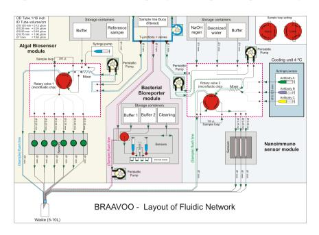
Figure 17 – General layout of the fluidic requirements of the three BRAAVOO biosensors.
